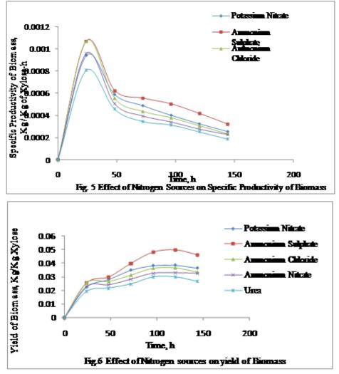
The work is extended by performing experiments with different concentrations of Ammonium Sulfate to know the optimum concentration of Ammonium Sulfate. Concentrations of 4, 6, 8, 10 g/l of Ammonium Sulfate are used in the experimental work wherein it was found that xylitol production is highest at 4 g/l of Ammonium Sulfate as seen from Fig. 7.
